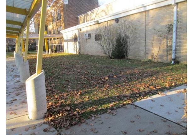
A bioretention system can be installed in the turf grass area near the entrance of the building capture, treat, and infiltrate rooftop runoff. The two downspouts in this area can be disconnected to direct stormwater from the building into the bioretention system. A preliminary soil assessment suggests that the soils have suitable drainage characteristics for green infrastructure.
