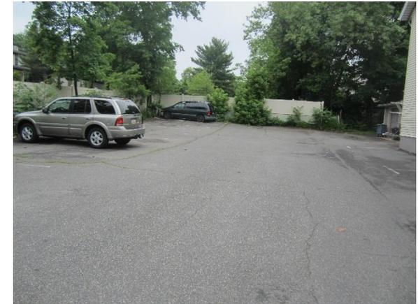
Parking spaces can be repaved with porous asphalt to infiltrate parking lot runoff. Downspouts on the northern side of the building can also be disconnected into rainwater harvesting systems. The walkway on the southern side of the building can be repaved with porous asphalt in order to better manage the stormwater from the building. A preliminary soil assessment suggests that the soils have suitable drainage characteristics for green infrastructure.
